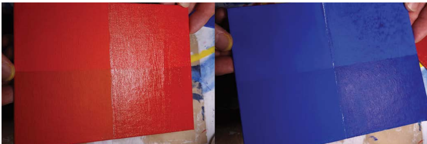
On the left is Naphthol Red Light, on the right Ultramarine Blue. A single coat of Golden SoFlat on the left of each canvas panel is compared with Golden Heavy Body on the right. The lower half of each panel is underpainted with Neutral Grey 6 to show the relative opacity.
