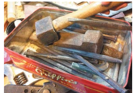
Some of Kap's tools, including chisels and his soft metal hammer, showing spread caused by banging.
