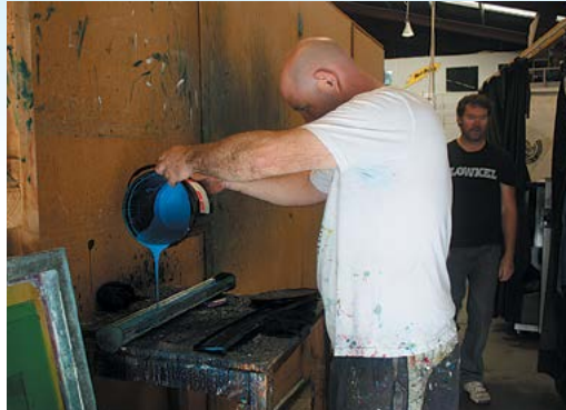
Here we see Reuben Ward, with Brett Sands in the background, pouring the emulsion which is coated onto the screen with a coating trough. The emulsion is light sensitive.
