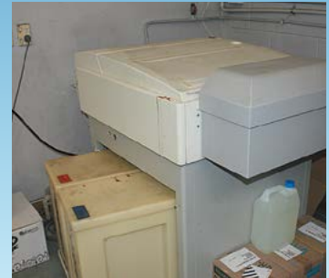
The film gets fed through the processor and developed. The outcome is a black image on clear film.
