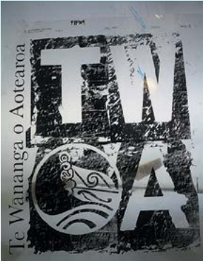
A picture of the film on the light table. Checks need to be completed to ensure the black is dense enough.
