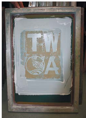
The above two pictures are of each side of the screen after it has been printed. A mirror image and a true image. The process doesn't end here. The screen needs to be reclaimed.
