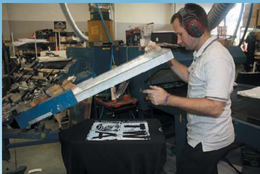
Checking to see the print is good, Jason will often print a white, flash dry then print again to ensure a dense coverage.
