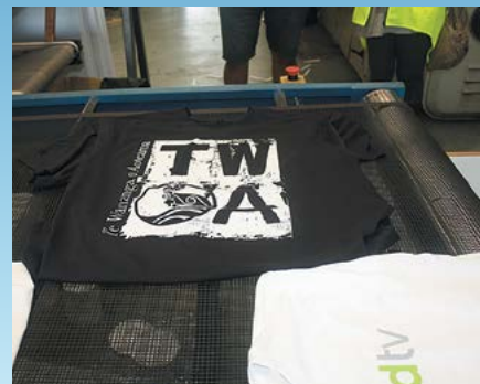
The T-shirt is placed on a belt that runs through a drying machine, sealing the ink.
