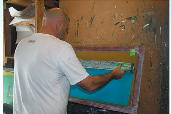
Reuben coats the emulsion on the screen, turning the screen around and spreading it on both sides. Once the emulsion is spread evenly, the screen is placed in a dark room to dry.
