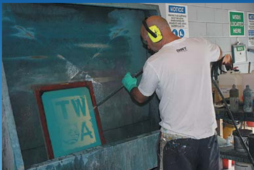
Reuben washes the screen, removing the emulsion that hasn't been exposed, creating the template for the screen print.
