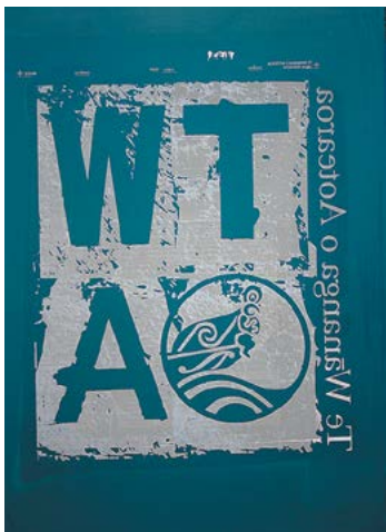
The above two pictures are of each side of the screen after it has been printed. A mirror image and a true image. The process doesn't end here. The screen needs to be reclaimed.
