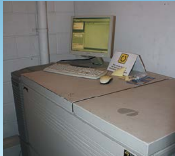
Once approved, the artwork is printed to an imagesetter onto light sensitive film that feeds into a light fast box.
