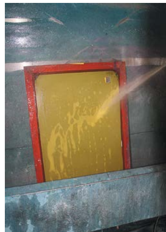
In the final step, various chemicals and a high pressure hose ensure the screen is thoroughly cleaned, degreased and ready to be re-used. ■
