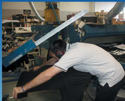
Jason Elson positions a T-shirt on the board after he has positioned the screen correctly. Precision is vital at this point.
