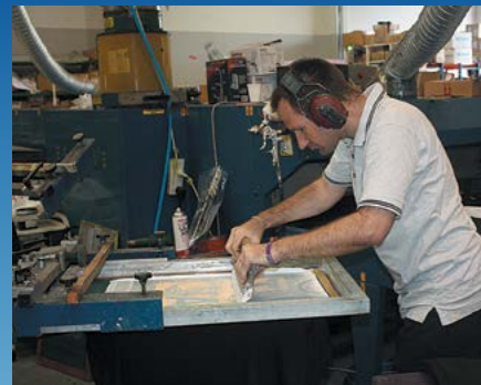
Jason uses a squeegee to pull the white printing ink over the screen, ensuring that even pressure is applied.
