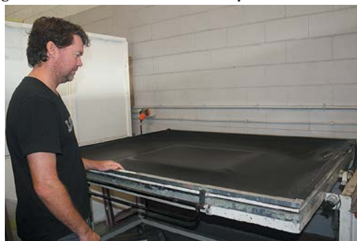
When the emulsion on the screen is dry, the film gets positioned carefully on the screen, and placed in a vacuum sealed frame with black fabric on one side and clear glass on the other. The vacuum ensures nothing moves inside the frame. Brett secures the frame and flips it over so the clear glass is facing forward. Then an ultraviolet light is shone on the glass (as seen right). This light burns through the clear film, hardening the emulsion. Any part of the screen that doesn't get light will wash clear.
