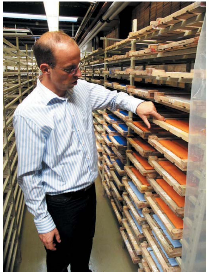
Markus Baumgart of Schmincke shows the Soft Pastels in the drying racks, waiting to be hand-wrapped.
