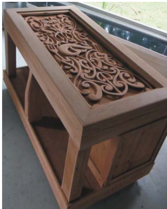
Kauri butchers block (on casters) nearly completed, carved slab is about 120mm thick and comes in at a mere 3,500 years old and the structural timber has been used from a wall borrowed indefinitely from our 100 year old house so heaven knows how old the tree was that that came from back in the day. Glass to insert on top when finished and LED lighting to highlight the carving from under the glass.
