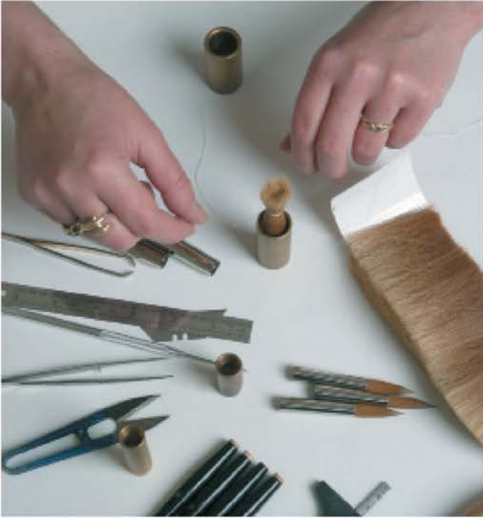
1. The amount of 'fill' is selected, placed in the goblet (sometimes called a brass cannon), and tied.
